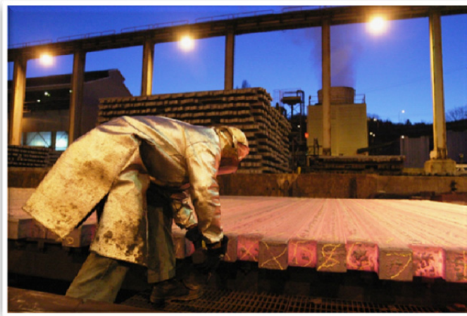
Steel billets roll red hot along the Nucor production line
